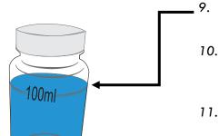
Fill the bottle to the 100mL line. Our laboratory will not accept sample less than 100mL.
