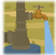
Pump water to waste sufficient volume to flush the spigot and lines (~5 to 10 min) before collecting sample.
